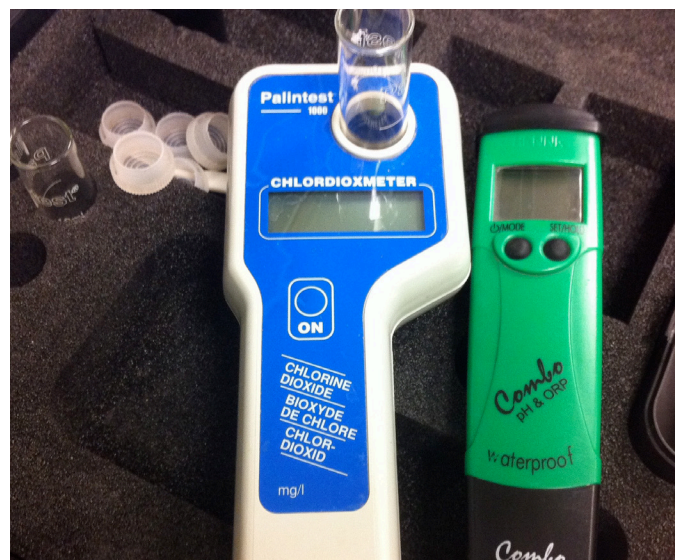
pH meter and CL meter
